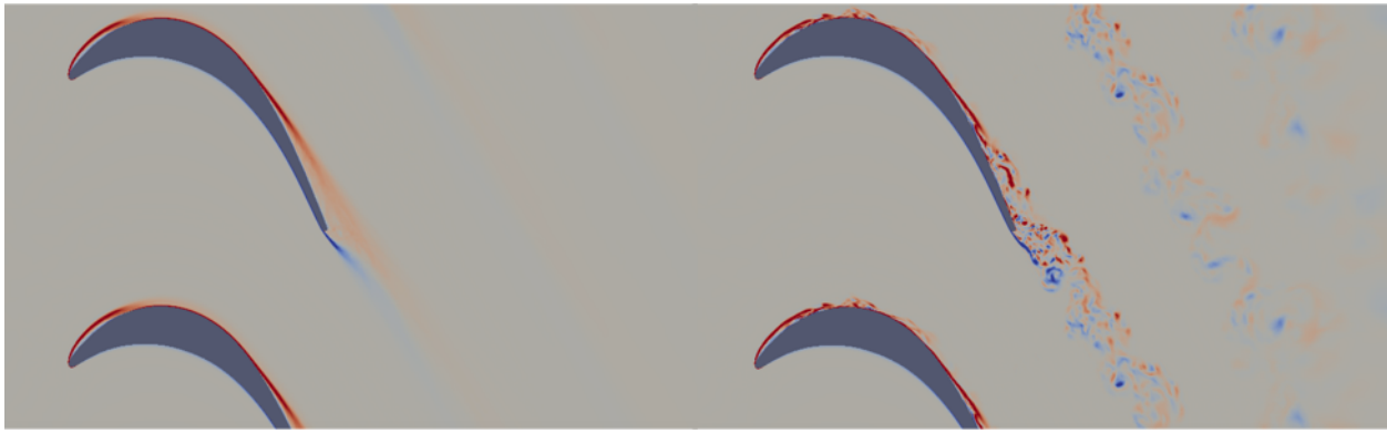
Figure 10: Time-averaged (left) and instantaneous (right) spanwise vorticity fields for the transonic T106C LPT. The shock capturing method seems to have little to no impact on the resolved vortical structures across the shock.
