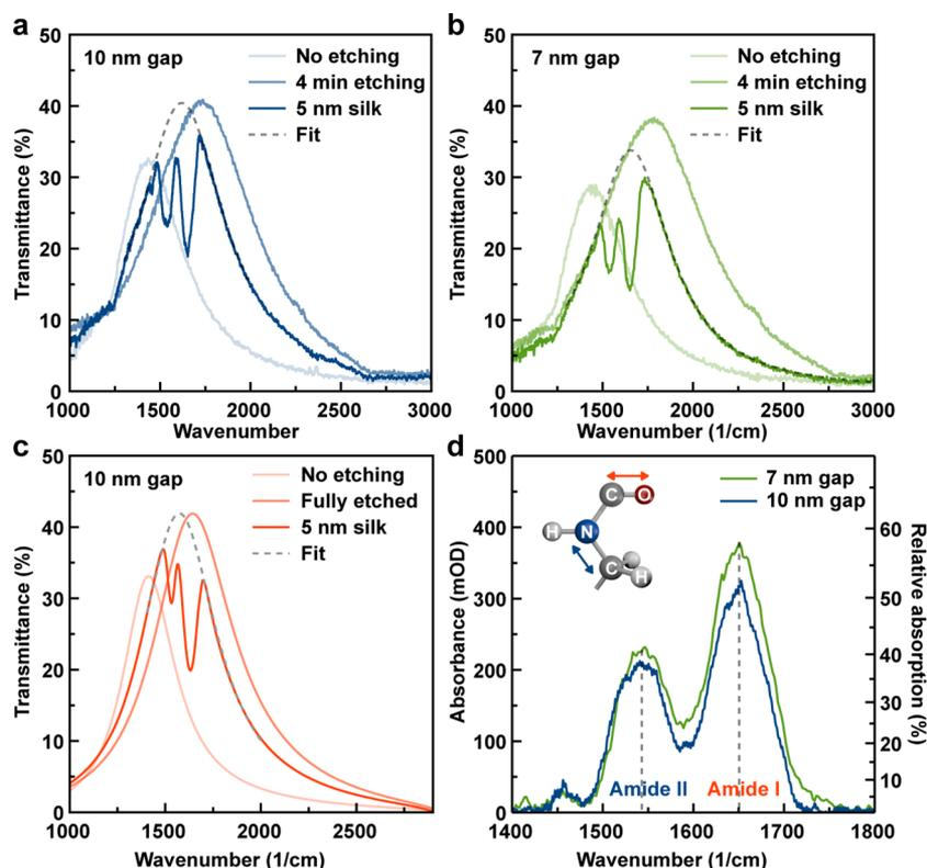
**Figure 4.** (a,b) The comparison of zero-mode resonances measured from 10 and 7 nm wide coaxial nanoapertures respectively, before  $\text{Al}_2\text{O}_3$  etching, after  $\text{Al}_2\text{O}_3$  etching, and after silk spin-coating. (c) The comparison of zero-mode resonances for each step numerically modeled using FEM. (d) Absorbance calculated from (a,b). Two distinct absorption signals resulting from the amide I and II bands of protein molecules are shown.
